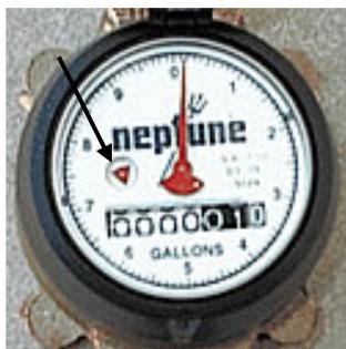
The “sweep indicator” is located to the left of the meter dial and will move when any water passes through the meter.
