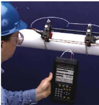
A well meter is tested using an ultrasonic clamp-on meter. Mastermeters can also be tested this way
